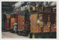
This impressive line of transformers nearing completion shows (right to left) 20,000 kVA Generator Transformer for the North of Scotland Hydro-Ellectric Board; 13,000 kVA unit for the British Ellectricity Authority; and a 4,575 kVA Mercury Are Rectifier Transformer for South African Railways.
