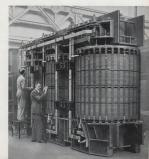
A 130-ton 75,000 kVA Generator Transformer, one of two built in 1949 for Portobello Power Station.
