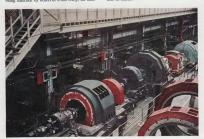
Main Testing Department showing (left to right):—10,000 kW hydro-electric generator for New Zealand; 1,900 B.H.P. a.c. motor for South Africa; 2,500 kW geared generator for Australia; 15,000 kVA synchronous condenser for New Zealand.
