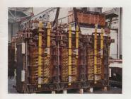
This 3-phase 33,000-volt Oll-Immersed Magnetically Shielded Reactor, one of four built in 1948 for Portobello Power Station, is believed to be the largest of its type to be built in Britain up to that time. It is designed to limit the short circuit current to 45,000 kVA.
