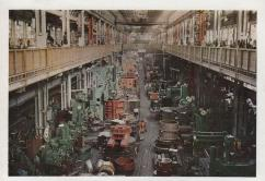
Main bay of Rotating Electrical Machinery Shop showing the diversity of the work undertaken. Flow of materials is undirectional, each process leading to the next. Components and sub-assemblies are dealt with in side bays and galleries.
