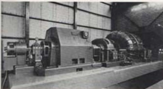
A 2900hp 1800rev/min synchronous motor driving a centrifugal blower at a Canadian nickel ore plant.
