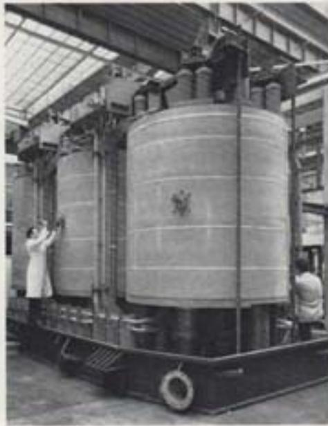
A 360MVA 230/500kV auto-transformer for a Canadian transmission substation on test at the Company's factory.
