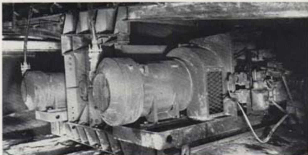
A 3.3kV direct-on flameproof starter for the control of a main conveyor belt motor-drive in a Canadian coal mine. Below, medium-voltage flameproof motor control gear installed in a British coal mine. In addition to controlling drill guns, conveyor motors and lighting, control is provided for Ambau Hobel equipment at the coal face.
