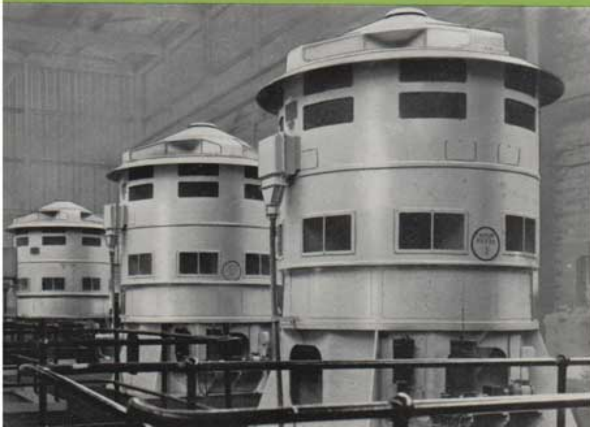
350 h.p. 1480 r.p.m. 3.3 kV closed-air-circuit air-cooled flame- proof squirrel-cage induction motor fitted with short-circuit- tested flameproof terminal assembly for a system fault level of 150 MVA
