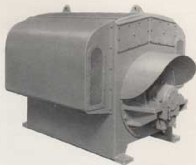
130 h.p. 585 r.p.m. 3.3 kV totally-enclosed fan-cooled flameproof squirrel-cage induction motor fitted with short-circuit- tested flameproof terminal assembly for a system fault level of 75 MVA
