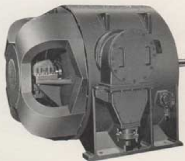
350 h.p. 1480 r.p.m. 3.3 kV closed-air-circuit air-cooled flame- proof squirrel-cage induction motor fitted with short-circuit- tested flameproof terminal assembly for a system fault level of 150 MVA
