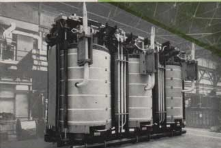
180 MVA transformer core and windings
