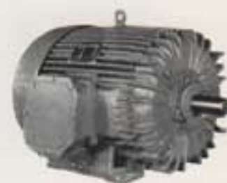
60 h.p. 2960 r.p.m. 415 V totally-enclosed fan-cooled squirrel-cage induction motor to the standard fixing dimensions of BS 2960
