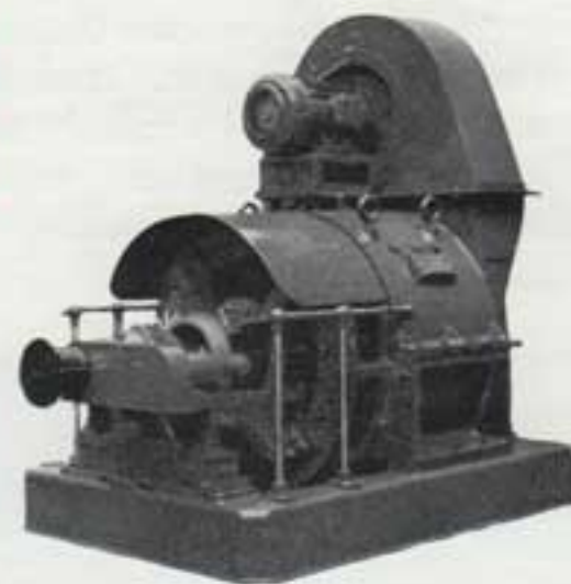
1500-580 h.p. 700 V 1550-600 r.p.m. pipe-ventilated forced-draught d.c. motor
